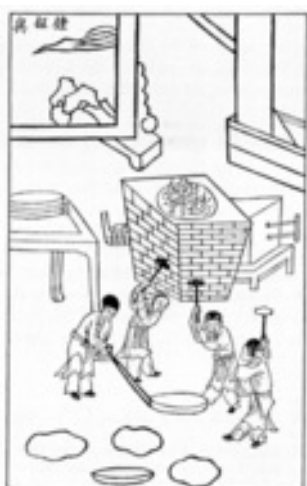
11. Drawing from the Tiangong kaiwu , Treatise of technology from the 17th century, and depicting the hammering of zhuo or tonggu
