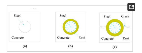
**Figure 3.** The corrosion process in the reinforced concrete; (a) without corrosion; (b) little amount of corrosion; (c) corrosion made concrete broken.
