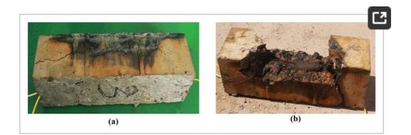
**Figure 21. (a)** the large cracks of specimen No.3; **(b)** Corrosion of the steel bar in specimen No.3.
