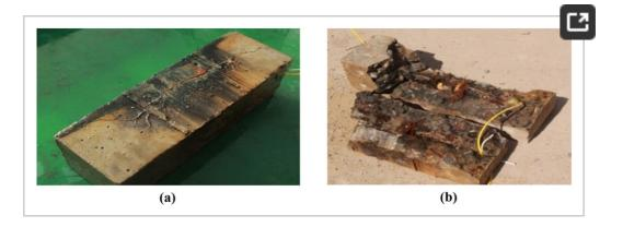
**Figure 24. (a)** The large cracks of the specimen No.4; **(b)** Corrosion of the steel rebar in specimen No.4.
