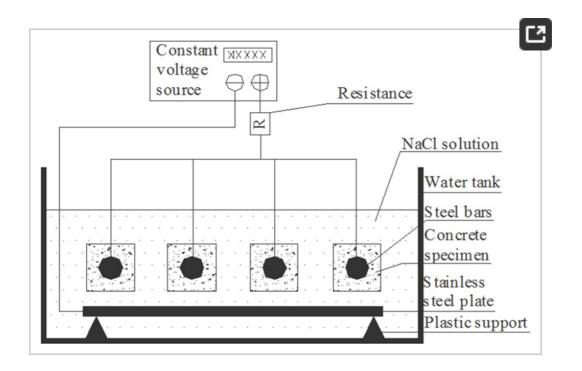
**Figure 8.** Schematic diagram of the electrochemical corrosion acceleration experiment system.
