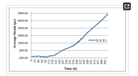
**Figure 19.** The average expansion strain result of S.3 (II).
