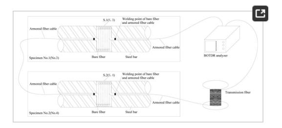
**Figure 10.** Fiber optic circuit of the corrosion monitoring experiments.
