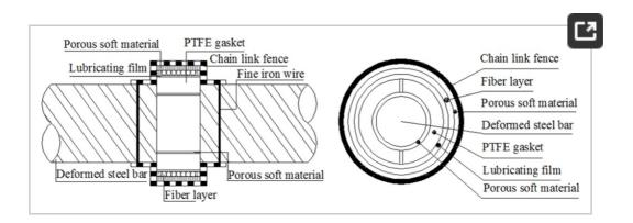
Figure 7. Packaging structure of BCES-III.
