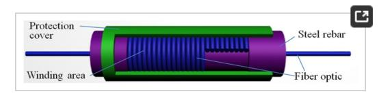
**Figure 4.** Basic packaging structure of the Brillouin corrosion expansion sensor.
