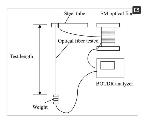
**Figure 2.** Setup of the strain calibration experiments.
