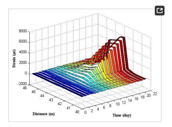
**Figure 18.** Corrosion expansion strain results of S.3 (II) in experiment two.
