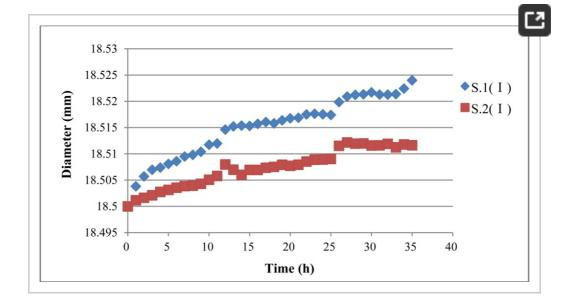
**Figure 15.** Steel rebar diameter monitored of sensor S.1 (I) and S.2 (I).
