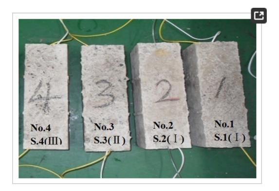
**Figure 9.** Concrete specimens with embedded sensors.
