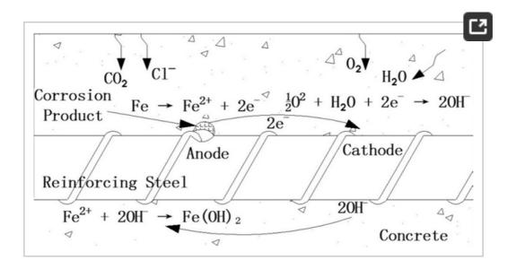
**Figure 1.** Schematic diagram of reinforcing steel corrosion in concrete as an electrochemical process.
