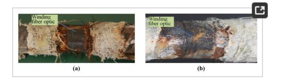
**Figure 17. (a)** The steel corrosion of S.1 (I) in the specimen No. 1; **(b)** The steel corrosion of S.2 (I) in the specimen No. 2.
